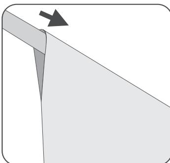
**5** If the banner is being hung by pole pockets, slide the horizontal support poles through the top and bottom pole pockets.
