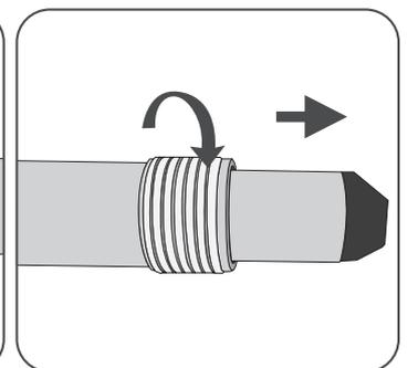
**4** Adjust the graphic width by rotating the pole extension locks to loosen the telescopic pole. Pull to the desired length, and gently tighten the pole extension locks. DO NOT over tighten pole extension locks.
