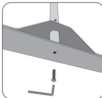
**2** Attach the vertical support poles to the feet using the bolts and screwdriver included.
