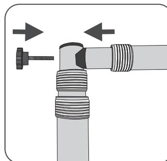
**6** Attach the horizontal poles to the vertical support poles using the large screws found in the end of each horizontal pole. Adjust the direction of the feet
