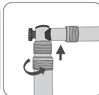
**6** Adjust the graphic height by rotating the pole extension locks to loosen the telescopic pole. Pull to the desired length, and gently tighten the pole extension locks. DO NOT over tighten pole extension locks.
